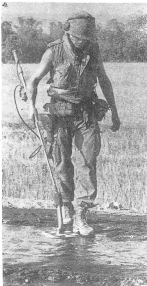
The operator swings the mine detector from side to side, followed by the prober who will investigate his findings. An hour often is required to cover a distance of a half mile. (US Army Photo by PFC Daniel Stroebel)
