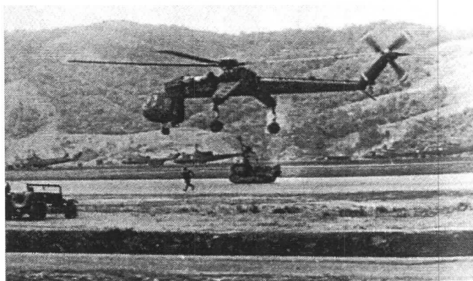
The flying crane lifts a bulldozer to the 101st in the Central Highlands province of Khanh Hoa, 197 miles NE of Saigon.
